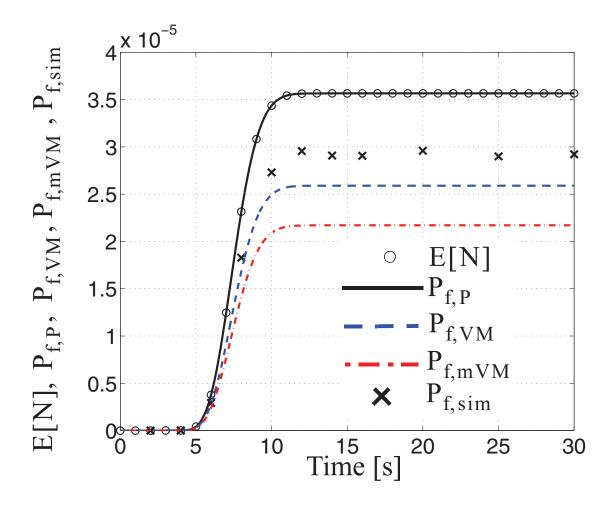
Table 1: Time-variant failure probability for linear elastic SDOF system with natural period  $T_0 = 0.5s$
